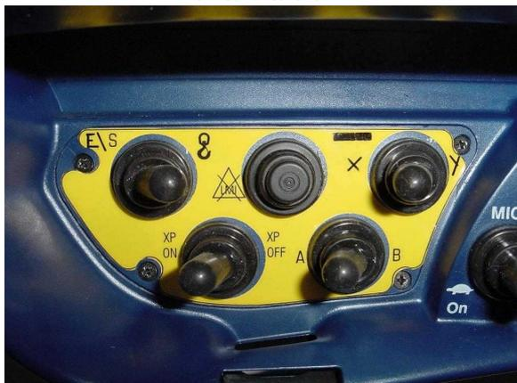
**XP** icon on the control handle of RCH radio controls
