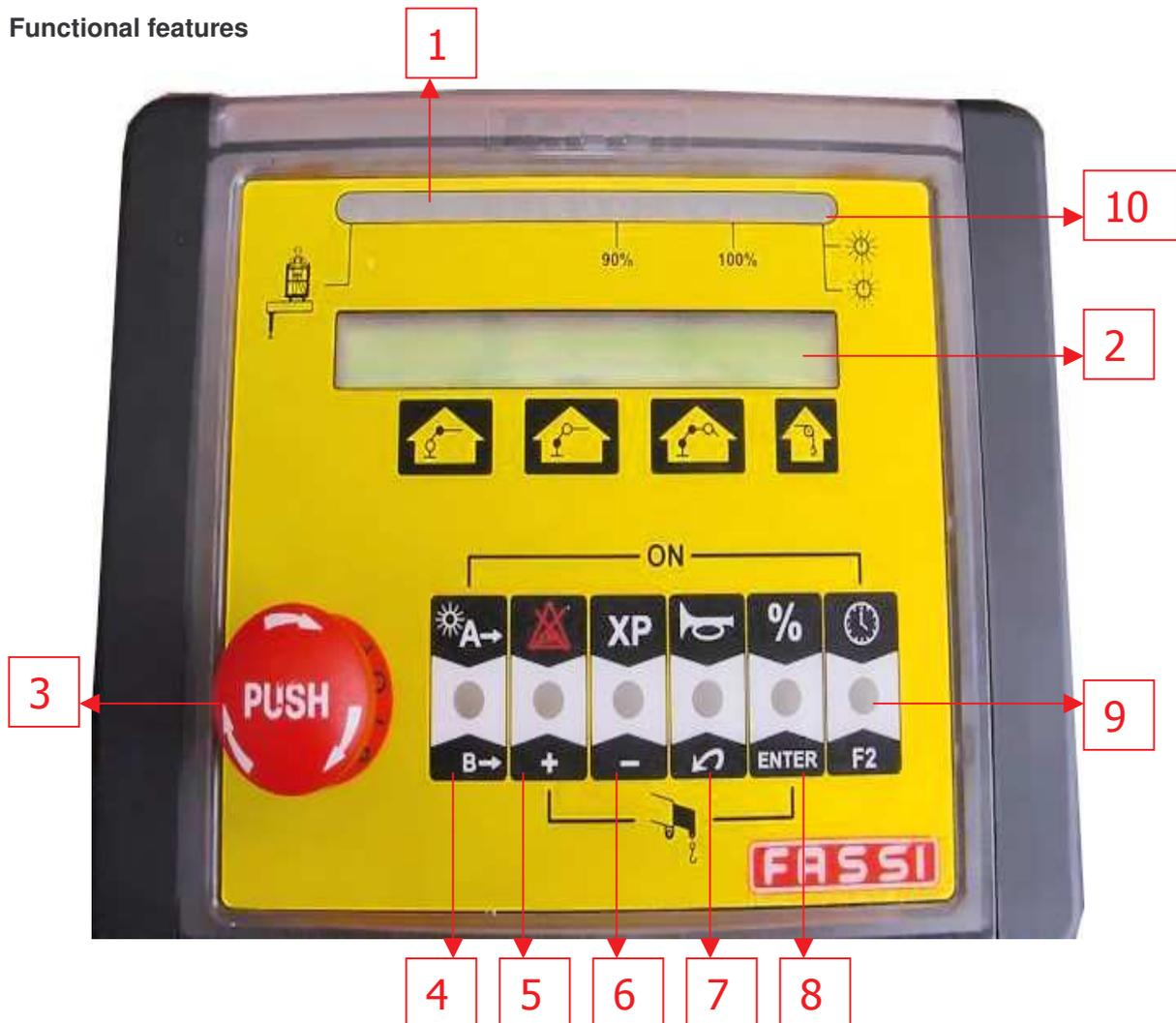
The panel includes a LED band indicator showing the percentage of load, an alphanumeric display, a series of buttons for menu navigation, the button for the activation of the acoustic signal, the button to activate the lifting moment limiting device exclusion (or alarm reset alarm), the XP device activation button and the emergency push-button.
